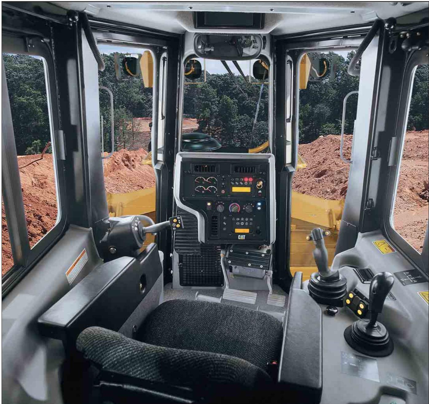
**Cab.** An isolation-mounted, pressurized cab reduces noise and vibration for operator comfort. The cab is pre-wired for a 12-volt or 24-volt radio, equipped with two speakers, an antenna and a radio mount recessed in the headliner.
