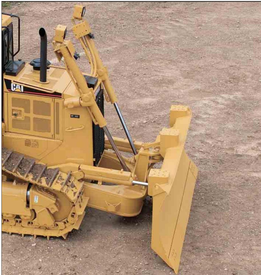
**Cat Blades.** All blades feature a strong box-section design that resists twisting and cracking. Blades are made of Cat DH-2™ steel that has high tensile strength and stands up to the most severe applications. Heavy moldboard construction and hardened bolt-on cutting edges and end bits add strength and durability.
