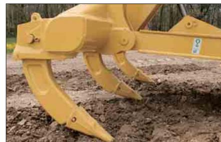
**Multi-Shank Ripper.** The multi-shank parallelogram ripper offers the choice of one, two or three shanks depending on job conditions. Curved or straight ripper shanks are available.
