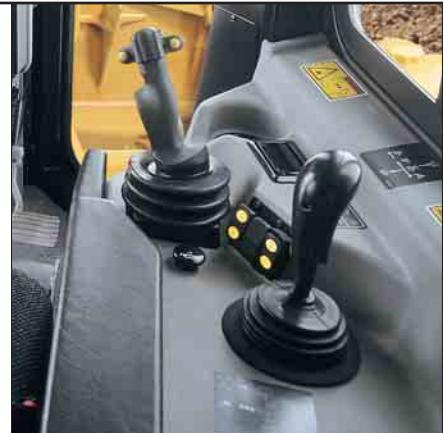
**Dozer Control Lever.** The D6R Series III features ergonomically designed dozer controls with low-effort, pilot-operated hydraulics for added operator comfort, easy operation and precise work tool control. When equipped with a VPAT blade, the blade control allows simultaneous six-way control of the blade with a thumb rocker control to adjust blade angle. The dozer control is changed to an electro-hydraulic control when the AccuGrade® Ready Option is installed.
