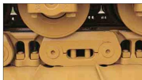
**Roller Design.** The SystemOne™ roller has a taller flange to improve track guiding, especially in side-sloping applications. Advanced features and reduced piece parts enhance the rollers which help eliminate any flexing in the collars and avoid oil loss. The roller is maintenance-free and serviced as a group only. To achieve total balanced wear, carrier rollers with increased wear life are also used.
