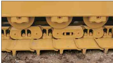
**Roller Design.** The SystemOne™ roller has a taller flange to improve track guiding, especially in side-sloping applications. Advanced features and reduced piece parts enhance the rollers which help eliminate any flexing in the collars and avoid oil loss. The roller is maintenance-free and serviced as a group only. To achieve total balanced wear, carrier rollers with increased wear life are also used.
