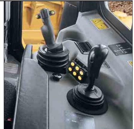
**Dozer Control Lever.** The D6T features ergonomically designed dozer controls with low-effort, pilot-operated hydraulics for added operator comfort, easy operation and precise work tool control. When equipped with a VPAT blade, the blade control allows simultaneous six-way control of the blade with a thumb rocker control to adjust blade angle. The dozer control is changed to an electro-hydraulic control when the AccuGrade® Ready Option is installed.
