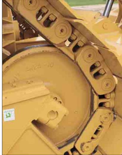
**Center Tread Idler.** The SystemOne Undercarriage uses center tread idlers which coupled with new, taller flange rollers, improve guiding and eliminate link scalloping. The center tread idler will increase system life 50 percent or more in most applications since they will last as long as two link assemblies. In combination with the rotating bushing design, the center tread idlers and sprocket segments can be reused through at least two undercarriage lives.
