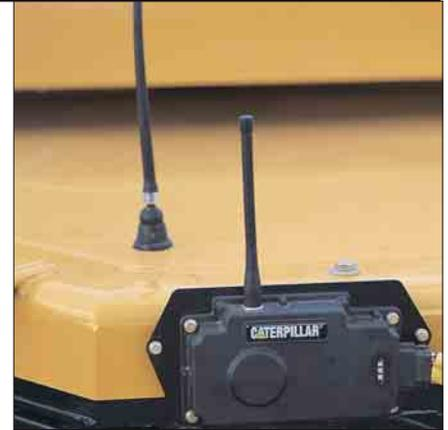
**Cat® Product Link.** When machines are operating at several different job sites, it becomes more difficult to keep current and accurate records. That can lead to missed maintenance, poor use of assets and wasted time. Product Link provides two-way information flow between machine on-board systems and your desktop computer through Dealer Store Front and Equipment Manager. Cat Product Link enables the use of Equipment Manager to keep you in touch with your machines.
