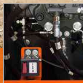
Primary filter head with ETP-Switch
